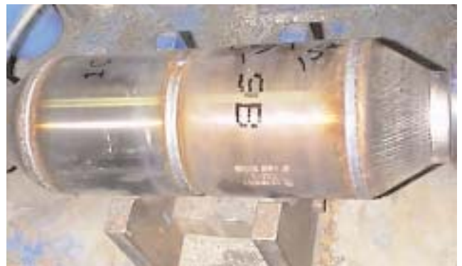
Hot end of an exhaust system in ferritic stainless steel.
